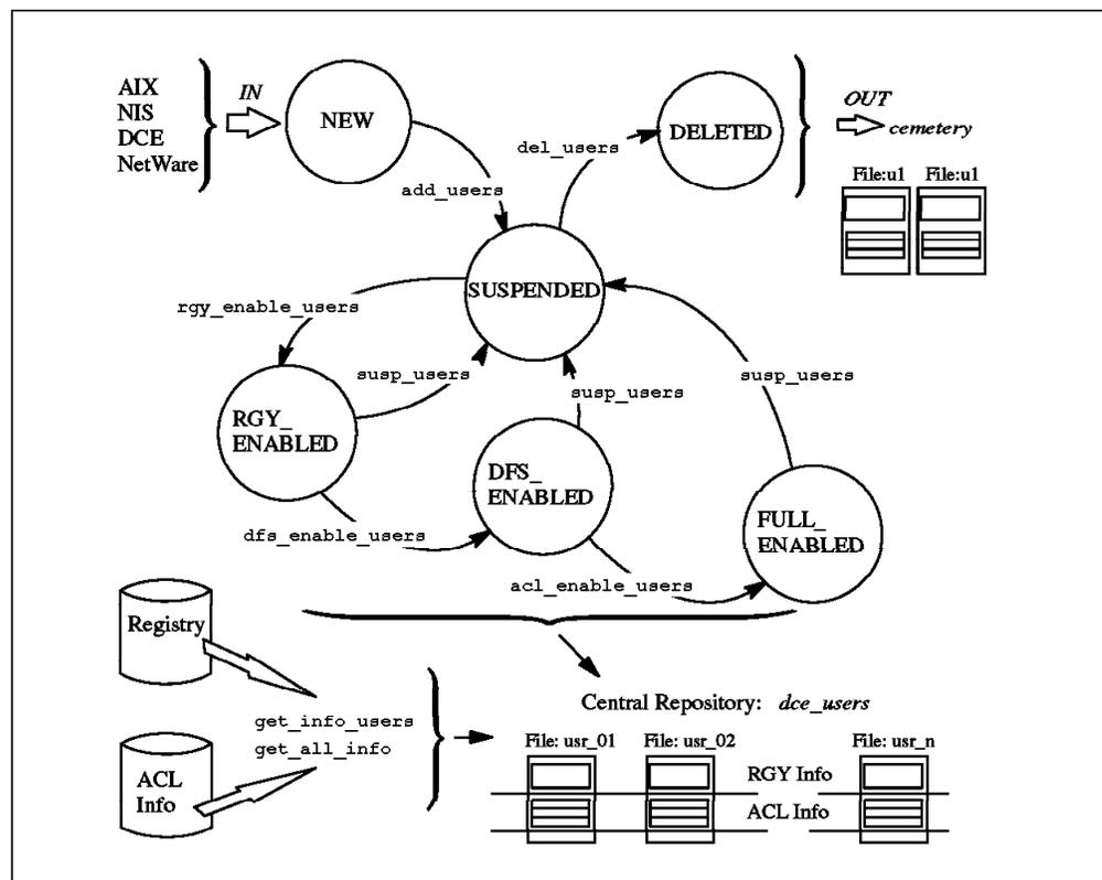
Figure 39. DCE User State Diagram. Each user defined with these set of tools is always in a certain state. The defined commands are used for state transition.
