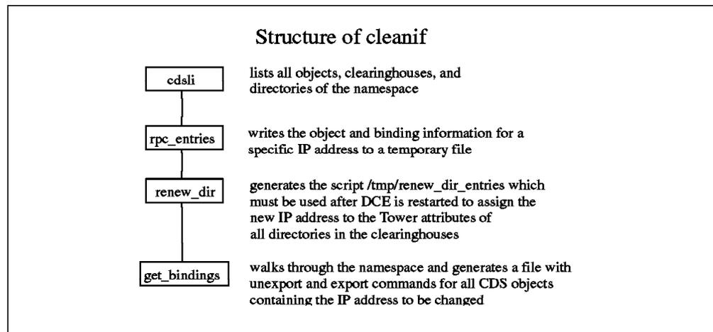
Figure 27. Workflow Description of the cleanif Procedure
