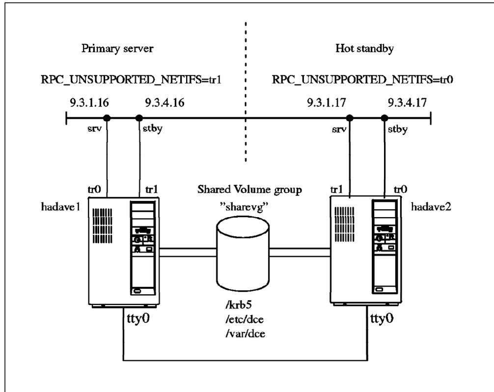
Figure 34. DCE on HACMP/6000. This cluster configuration was used with nodes `ev1`, `ev2`, `ev3`, and `ev4` (see scenarios in Chapter 3, "Implementing DCE Cells" on page 43), which were all defined as DCE clients.
