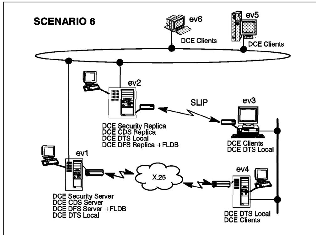
Figure 24. Scenario 6: A Branch Connected with Two Links
