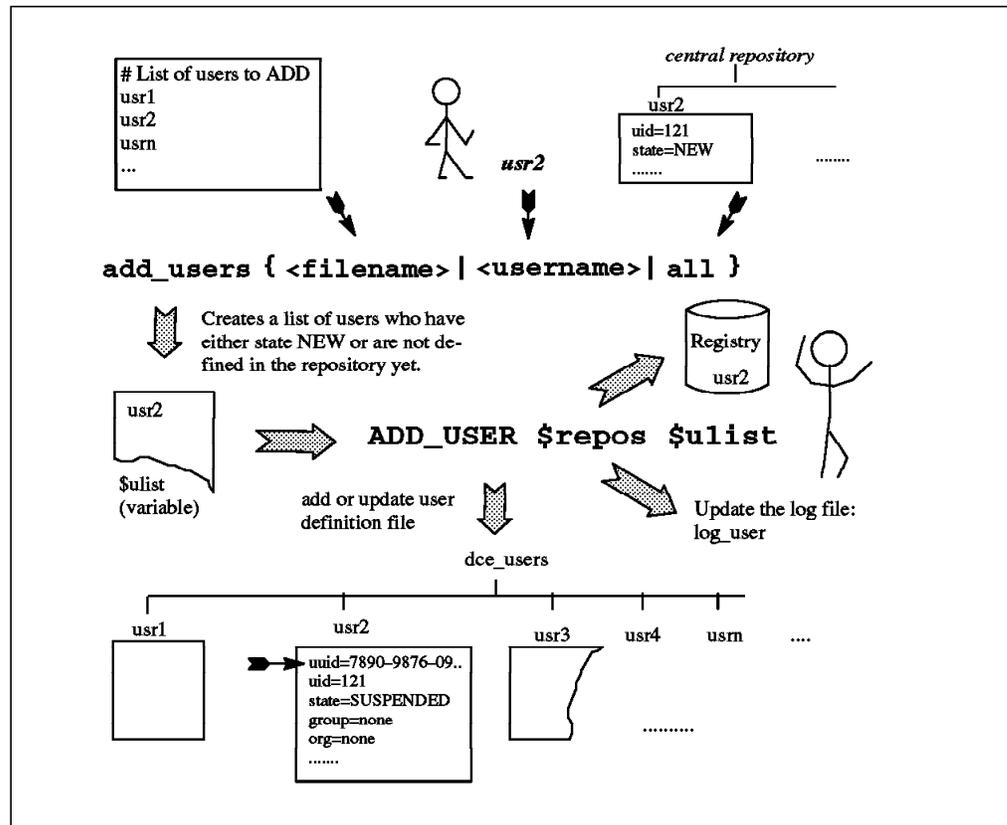
Figure 41. The `add_users` Procedure. After checking that the state of all candidates are `NEW`, the script `ADD_USER` is called, which creates entries in the DCE registry and in the central repository.
